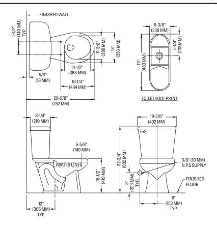
Fixture performance and specifications meet or exceed ASME A112.19.2-2013/CSA B45.1-13 standards, and other state and local codes.
