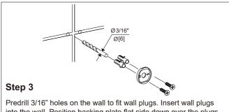
into the wall. Position backing plate flat side down over the plugs and install screws.
