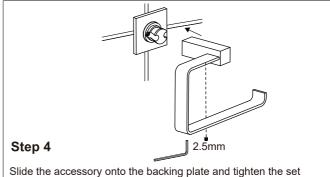
Slide the accessory onto the backing plate and tighten the set screw using Allen key provided.
