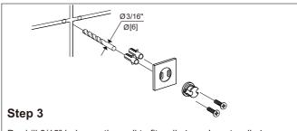
Predrill 3/16" holes on the wall to fit wall plugs. Insert wall plugs into the wall. Position backing plate flat side down over the plugs and install screws.
