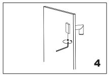
Fix the set screw on the end cap,tighten it to avoid loose from fixing brackets.
