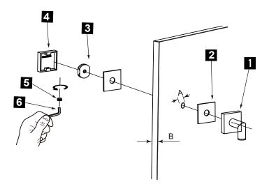
1.Knob x 1 2.Clear Gasket x 2 3.Fixing Bracket x 1 4.End Cap x 1 5.Set Screw M5 x 1 6.Allen Key 2.5mm x 1
