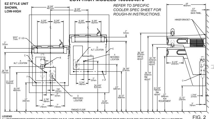
A = RECOMMENDED WATER SUPPLY LOCATION 3/8 O.D. UNPLATED COPPER TUBE CONNECT STUB WITH SHUT OFF (BY OTHERS) 3 IN. (76mm) MAXIMUM OUT FROM WALL PLATE.
