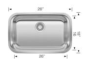
Undermount installation only Minimum cabinet size: 33" Cut-out Dimensions: Cut-out Length: 26.25" Cut-out Width: 16.25" Cut-out Below Counter Depth: 6.29" Bowl Dimensions: Bowl Length (left-to-right): 26" Bowl Width (front-to-back): 16" Bowl Width (front-to-back): 16" Bowl Depth: 5.5" Drain hole compatible with 3.5" strainers or waste flanges Nested SKU: 519435 Codes/Standards: ASME A112.19.3-2017/CSA B45.4-17
