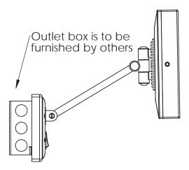
The center of the mirror is 7/8 " above the center of the outlet box. Since the typical user's eye height is 58 3/4" the outlet box should be centered 57 7/8" above the floor
